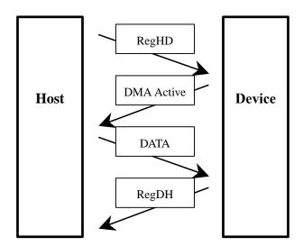
Figure 5.17 DMA data-out command protocol
